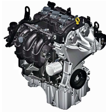
Figura 1.2: Motor Ford 1.0 TiVCT.
