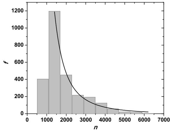
**Fig. 4.** The frequency ( $f$ ) of vehicle demand ( $n$ ) by using the ferry-boat system (gray bars). The black curve is the stationary solution of the nonlinear Fokker–Planck equation, i.e. a  $q$ -exponential curve.
