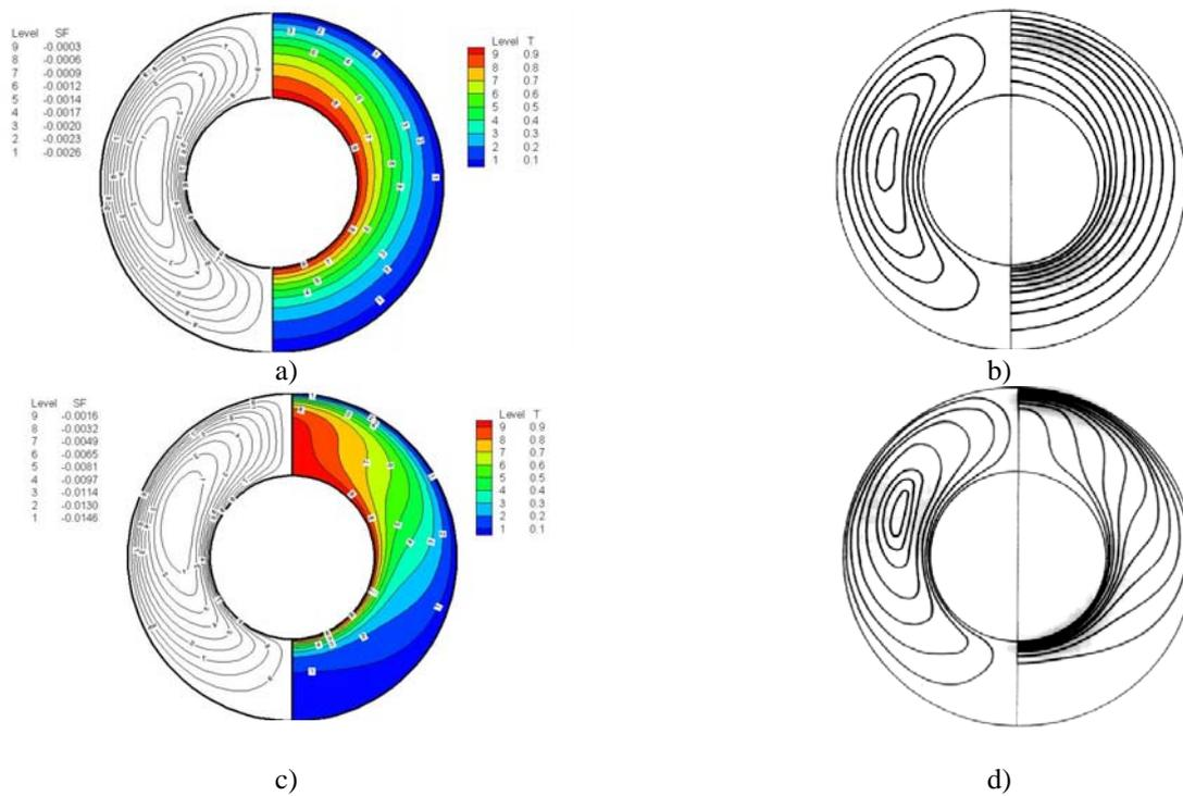
Figure 2. Laminar Isotherms and Streamlines for  $Ra_m = 25$  and  $Ra_m = 200$  with  $\phi = 0,2$ ,  $D_p = 3mm$  and  $r_o/r_i = 2$ ; a), c) Presents Results,  $N = 0$ ; b), d) Caltagirone (1976), ( $N = 0$ ).
