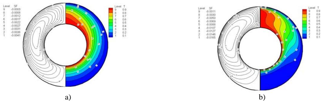
Figure 3. Laminar Isotherms and Streamlines for  $Ra_m = 25$  and  $Ra_m = 200$  with  $\phi = 0,2$ ,  $D_p = 3mm$  and  $r_o/r_i = 2$  with  $N = 1$ .
