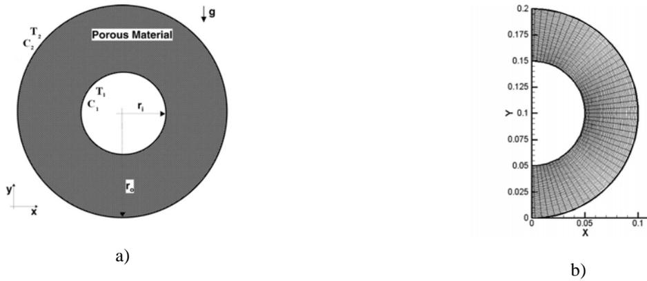
Figure 1. Schematic of the problem: a) geometry; b) grid.
