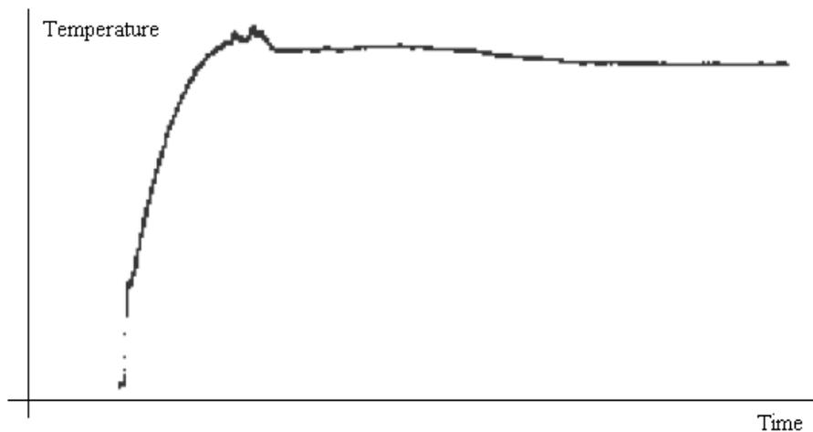
(b) Power[kW]= 1.16; y[mm]=3.0; dimensionless position=0.02; air dragging
