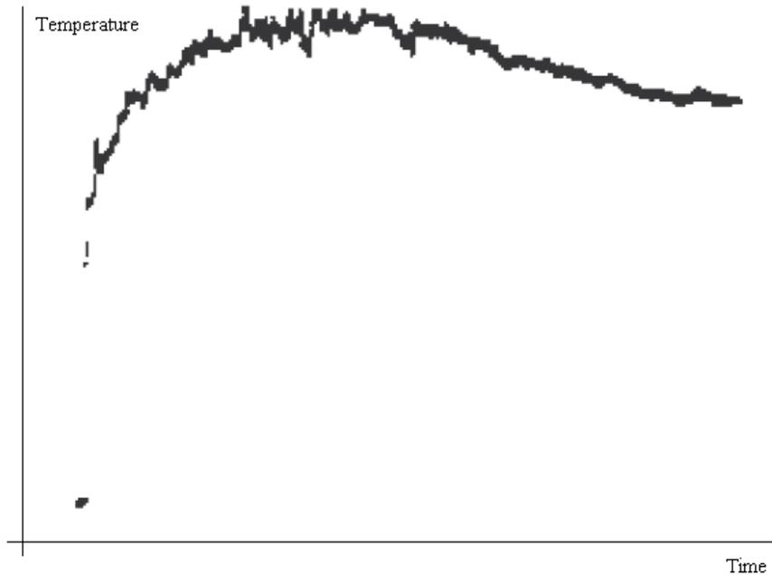
Figure 4. Temporary Variation of the Thermocouple Reading with Greater Soot Formation in the Region 1
