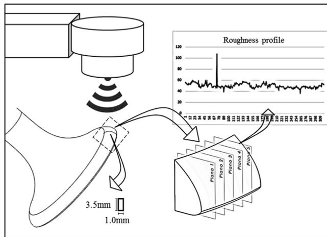
Fig. 4. 3D and 2D roughness profile capturing sequence.
