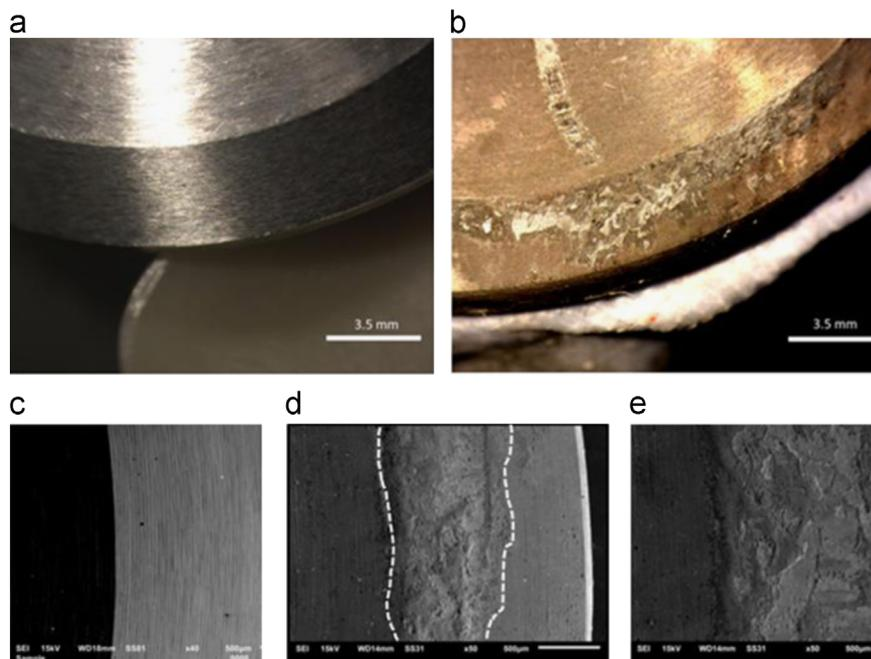
**Fig. 7.** Microscopy analysis on valve's surface before and after the tests showing additional material attached to the surface of the valve.
