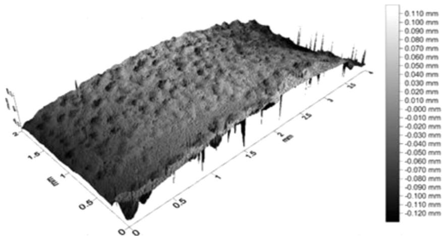
Fig. 5. 3D roughness profile obtained by optical profilometer from the contact surface of the valve subjected to 750 °C and a load of 6 kN.
