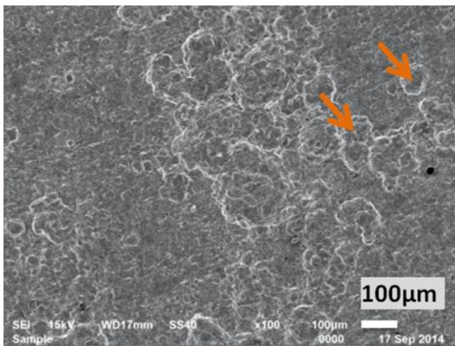
**Fig. 6.** SEM micrography of a valve surface tested at 750 °C under a load of 6 kN after 844,000 cycles.
