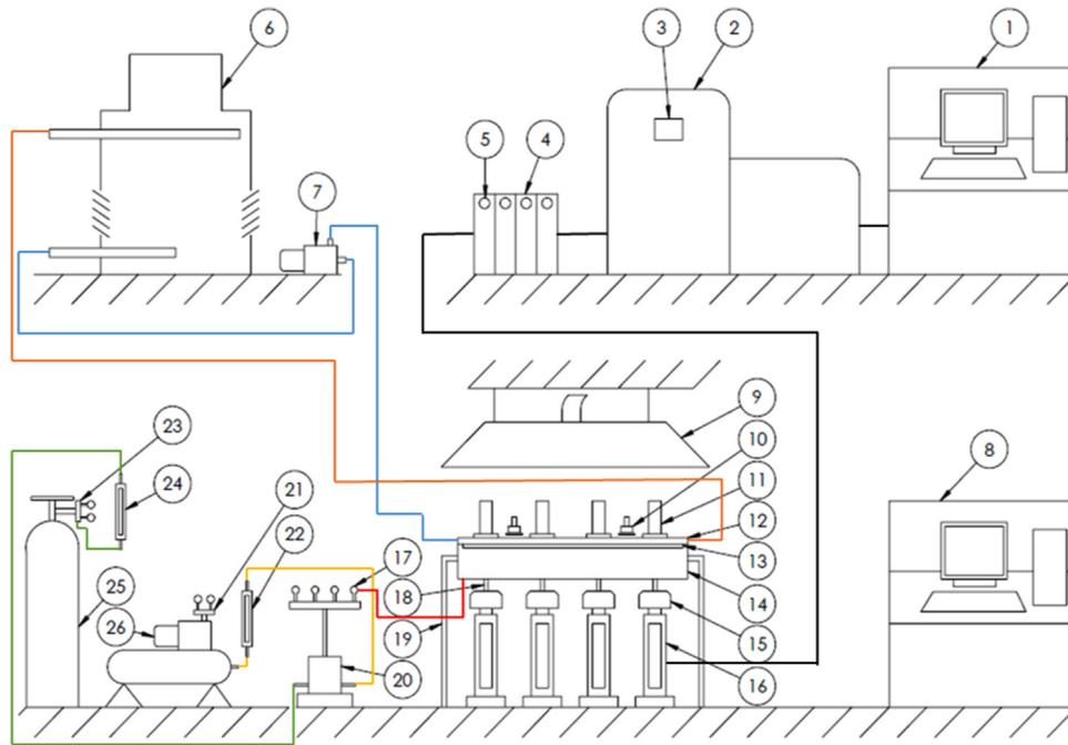
Fig. 1. Design layout of the wear test apparatus.
