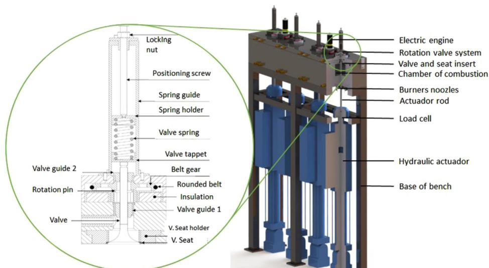
**Fig. 2.** General setup of the wear test apparatus used for testing the wear on the valves and, detailed in the bubble, the valve seats and the valve loading system.
