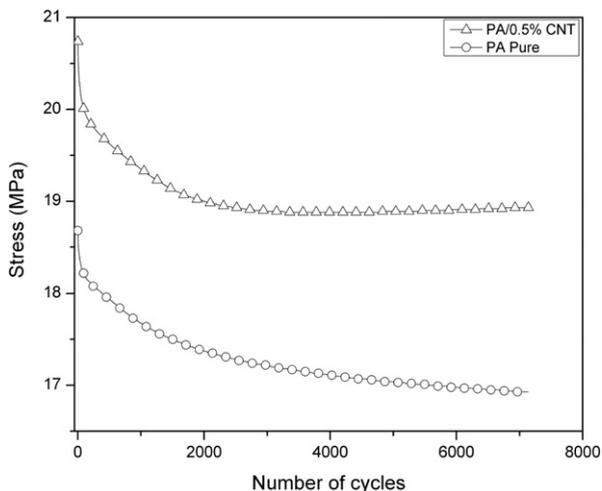
Fig. 7. Fatigue strength as a function of cycle number for PA and PA/MWCNTs composite.
