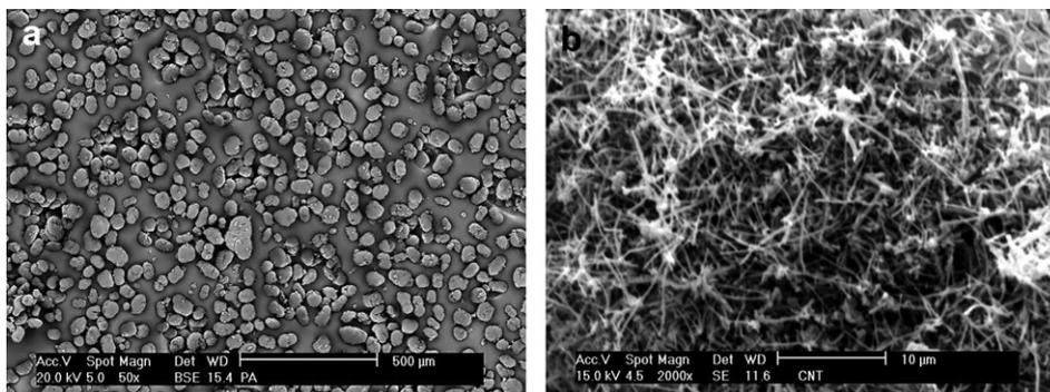
Fig. 1. Micrographs of PA12 particles (a) and MWCNTs (b).
