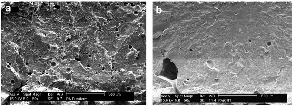
Fig. 5. Micrographs of cryogenic fracture surface of PA12 (a) and PA12/MWCNTs composite (b).
