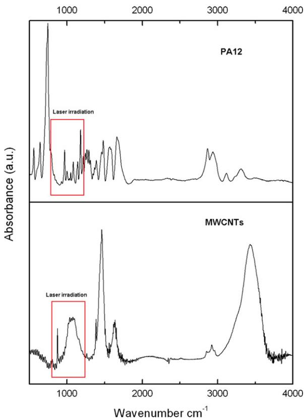
Fig. 3. Infrared spectra of PA12 and MWCNTs.
