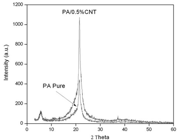
Fig. 4. X-ray diffraction patterns of PA12 and PA12/MWCNTs composite.
