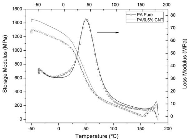
Fig. 6. Storage ( $E'$ ) and loss ( $E''$ ) moduli as a function of temperature for PA12 and the PA12/MWCNTs composite.
