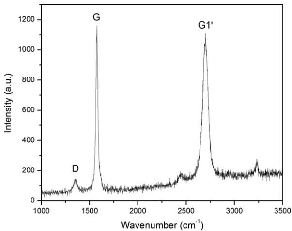
Fig. 2. Raman spectrum of MWCNTs.
