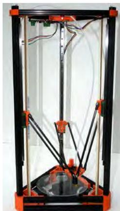
Figura 5. Impressora 3D Kossel (RepRap, 2015).
