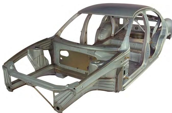
*Figura 7. – UltraLight Steel Auto Body Steel – ULSAB [9]*
