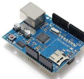
Figura 4 – *Ethernet shield*.
