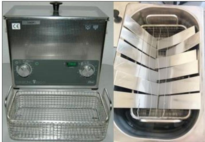
The first cleaning lasted for five minutes at room temperature of 23 °C using the ultrasound cleaner 460/H, from the company Elma Transsonic, shown in Figure 26, using a frequency of 35 kHz. The ultrasound cleaner removes dirties, particles, oil and greases, by creating micro bubbles that apply a very high pressure over the surface of the adherends, known as micro cavitation.
