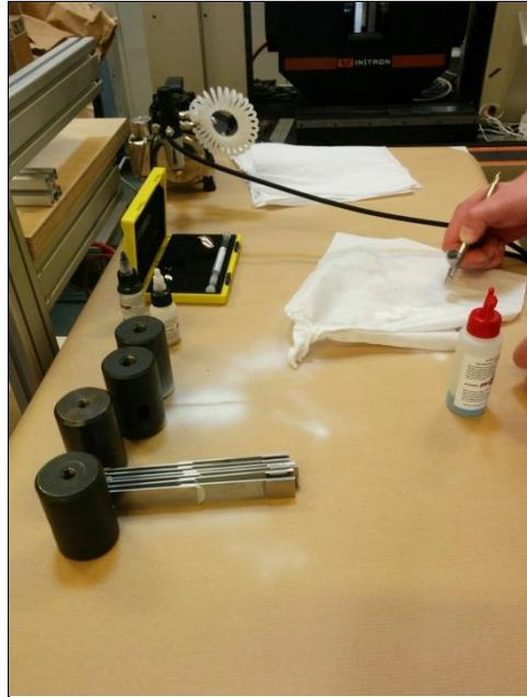
The result was a contrast between the two colors over the area of interest, which also blocks the reflection of the metal adherend, what would result in bad images. Prior to the test, the DIC cameras identify each point of the analyzed region. Figure 36 presents one prepared sample being visualized by the DIC system at the ISTR4 4D software screen.
