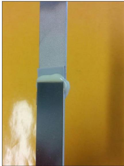
The excess of adhesive, shown in the sides of the overlap area of Figure 32, was removed from the sides with the usage of a grinder in order to avoid kame the load path uniform. The samples were then ready for the tensile tests, however, as mentioned in the beginning of this chapter, DIC analyses were also performed. So, a specific preparation was performed in order to accomplish this technique and will be explained in the next topics.
