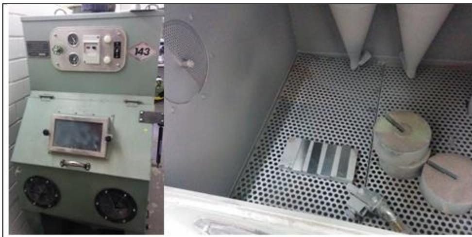
After the sandblasting it was used compressed air at 3 psi to remove the residual particles from the surface and also a tissue with isopropanol. After that a second cleaning was performed in the ultrasound cleaner for five more minutes with the same parameter of the first one, when the already abraded adherends are left there for five more minutes. After the second cleaning, a special care was taken with the prepared area in order to preserve a high surface energy from the treatment. So it
